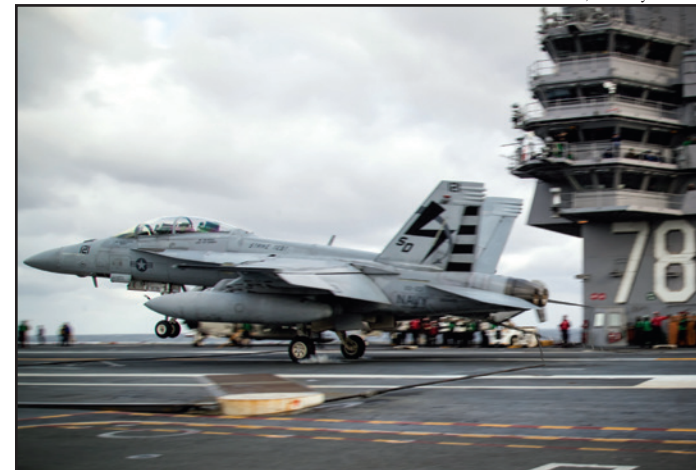
Above: A heavily laden VX-23 Salty Dogs F/A-18F Super Hornet recovers on board Ford, 17 Jan '20. Unlike on board Nimitz-class carriers, the arresting wires are directly adjacent to the island.
