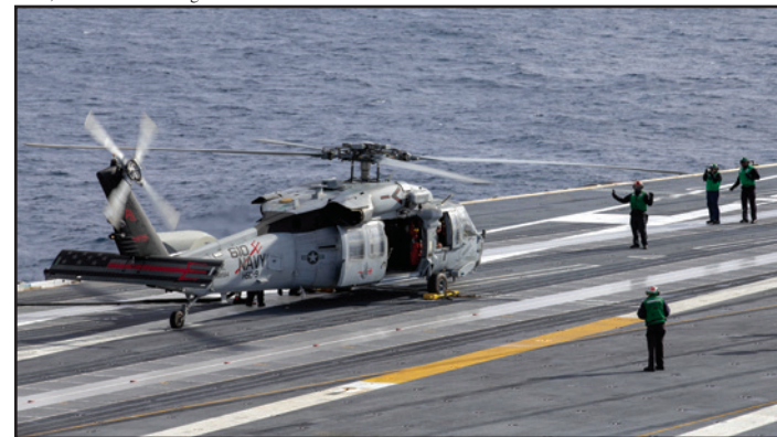
Air department Sailors refuel a HSC-9 Tridents MH-60S Seahawk on board Ford, 18 Jan '20. The flight-deck fuel stations are better situated for rapid aircraft turn-arounds.
