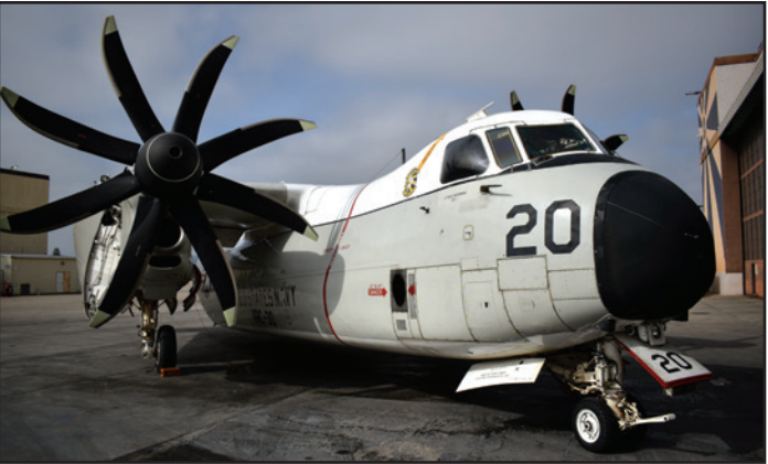
The C-2 with upgraded eight-blade propellers and avionics. The Greyhound has delivered exceptional service during its 58 years with the fleet.
