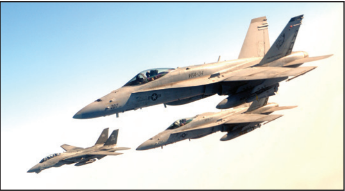
Hornets and Tomcats often flew mixed sections during Enduring Freedom and Iraqi Freedom. F-14s typically used their more advanced LANTIRN to laser designate for Hornets to deliver laser-guided munitions.
