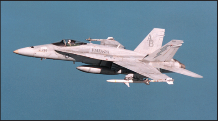
Many Operation Southern Watch patrols involved Hornets like this one from VMFA-251 carrying AGM-88 HARMs for potential use against Iraqi radar or SAM installations, and two AIM-9 Sidewinders for self-protection. A FLIR is visible on fuselage station 4.
