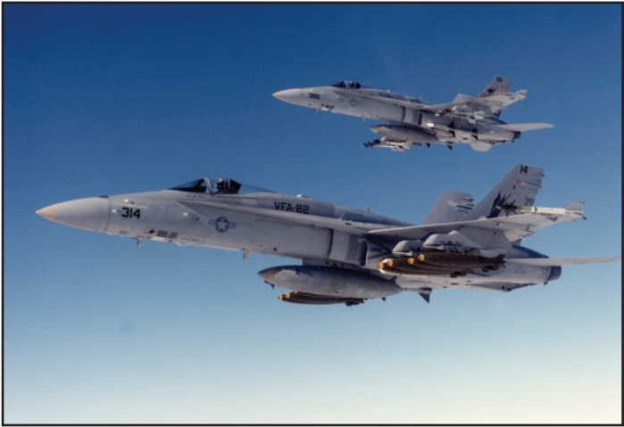
F/A-18Cs from the VFA-82 Marauders pictured in April 1989, one with a traditional strike load of eight Mk 83 1,000-lb. iron bombs and one with an air-to-air load of six AIM-9 Sidewinders and two AIM-7 Sparrows.
